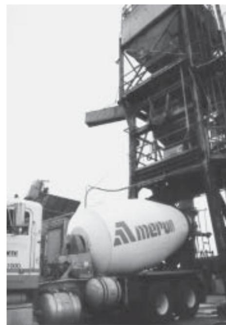
Dry cement is mixed with water in huge towers before being funneled into waiting cement trucks.
