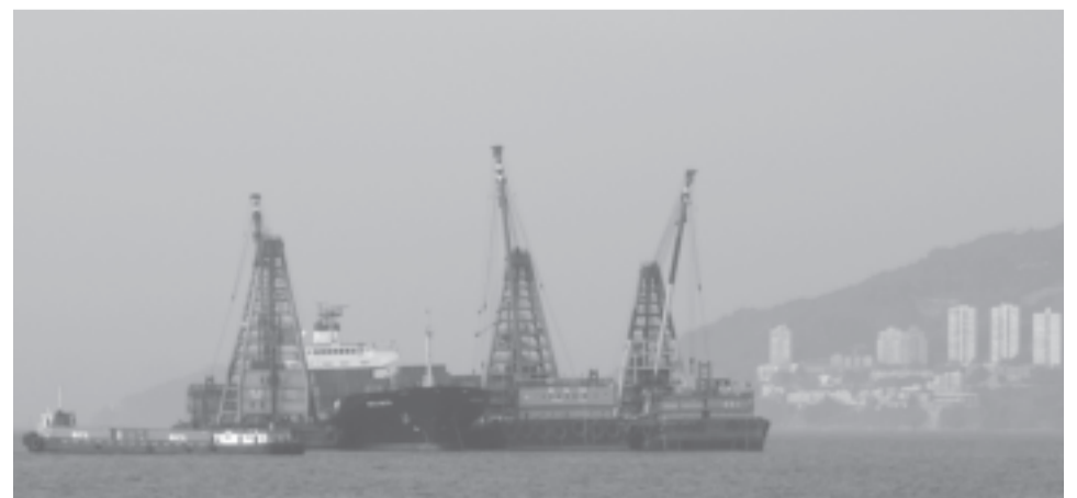
A dozen of these floating cranes in the middle of Victoria Harbor off the Island of Hong Kong transfer shipping containers from freighters to barges. Mid-stream operations where cargo is moved between two ships at sea avoids the high fees charged by the Hong Kong container port but can be dangerous and risky.
